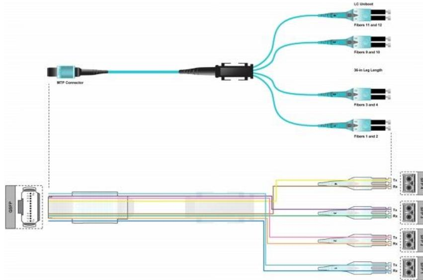
**Figure 5 - Example - Fan Out Cable**
